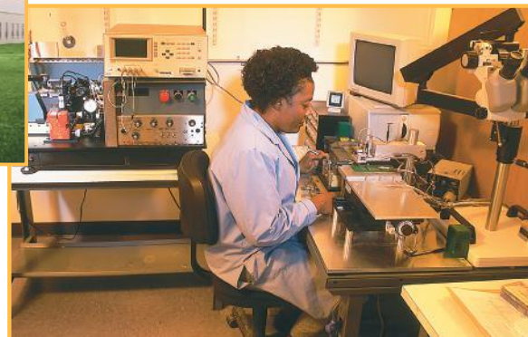
Autopacking center ► packages chips into waffle packs
