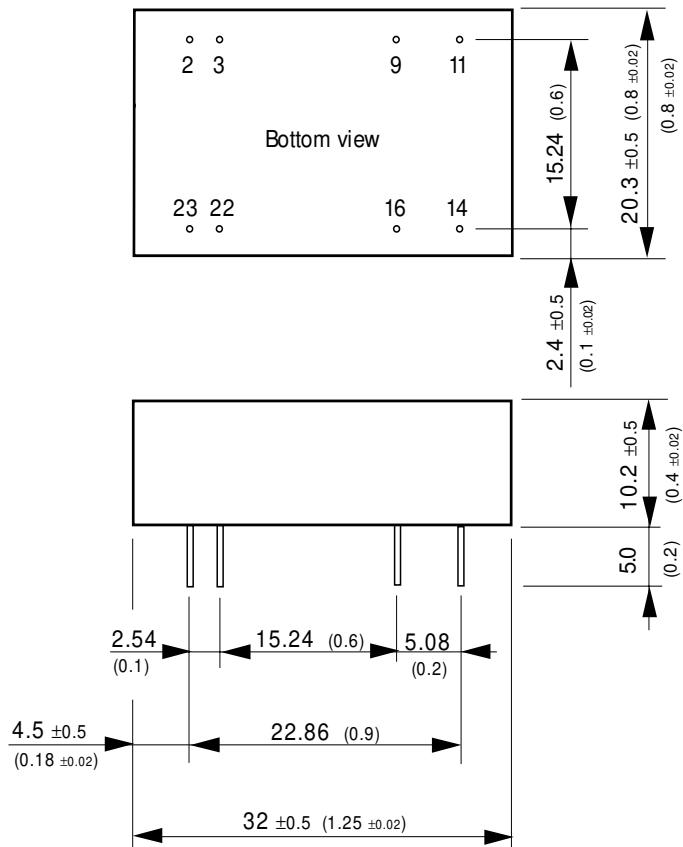
Pin diameter  $\varnothing 0.5 \pm 0.05$  (0.02)  $\pm 0.002$
